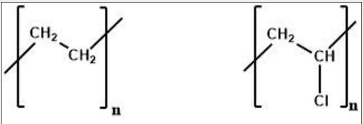
Figure 3 Structures of Polyethylene (HDPE and LDPE, Left) and Polyvinylchloride (PVC, right).
